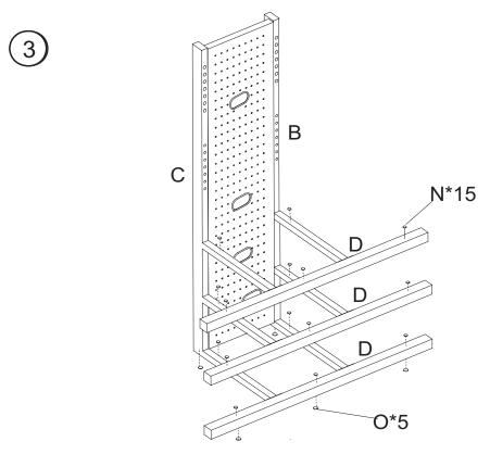
3-Place pads (N) on the beams (D) and frames (B & C). Apply pads (O) at the bottom of the unit.
